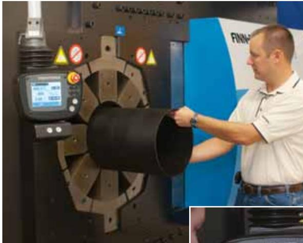
*The King Crimper 1200 features a new UC Controller, which has computing power and features never seen before on crimping machines, such as automated quality control reporting options and an easy to use menu guided operation.*
