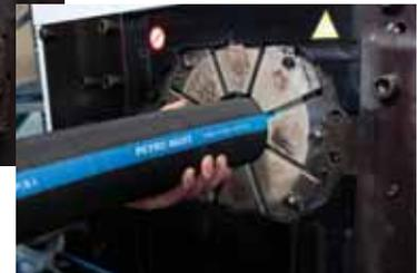
The FP160's wide opening is also a notable feature, according to Wickham. "We're not just able to do the 6 inch...we can open the dies quite wide so that we are able to get large end fittings through it without having to worry about running the whole length through," says Wickham.
