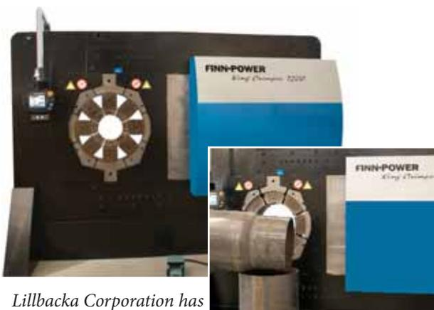
*Lillbacka Corporation has recently introduced the world's largest crimper, the King Crimper 1200. The King Crimper has a maximum crimping force of 1,200 tons and a crimping range from 7.87" to 25.59".*
