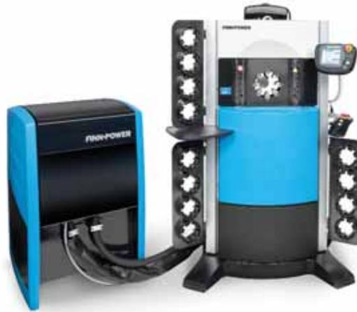
*These production units can accommodate both small and large assemblies. Their pass-through head design makes them ideal for crimping elbow assemblies, flanged pieces, and oddly-shaped parts.*
