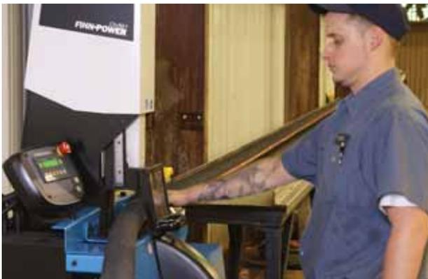
*Finn-Power hose cutting machines are also very popular at HosePower because they cut straight without burning the wire.*
