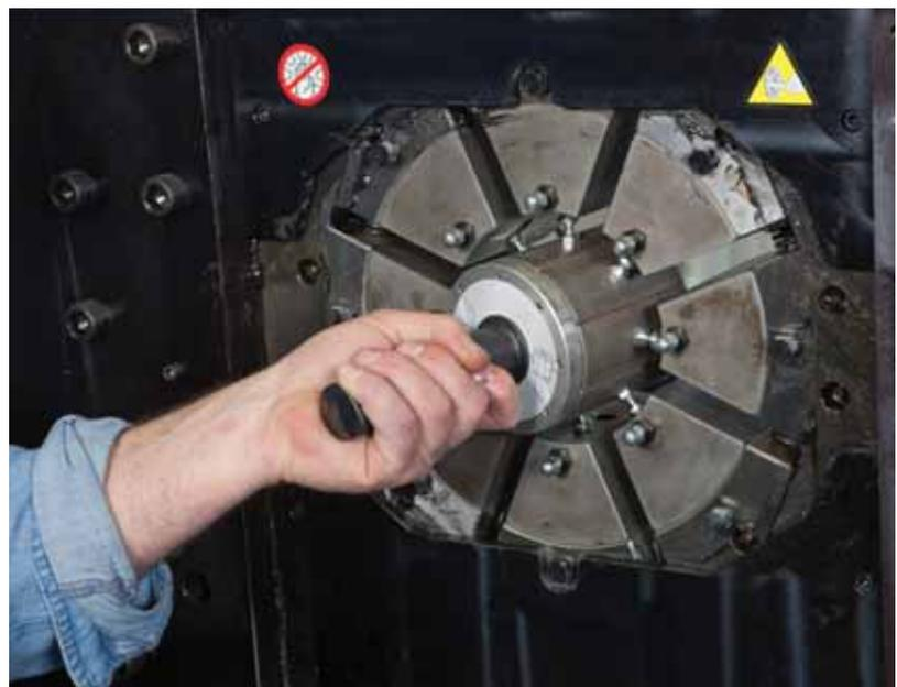
The Quick Change Tool System (QC) allows the entire die set to be changed in one easy operation. The pins on the QC Tool engage the QC holes in the dies. As the master dies open/close, the die segments are released from the master dies and retained by the QC tool. The die segments are held to the tool by a magnet. The die set then can be stored in the QC storage rack. In this way, the segments are kept in complete sets and are always used in the same order.
