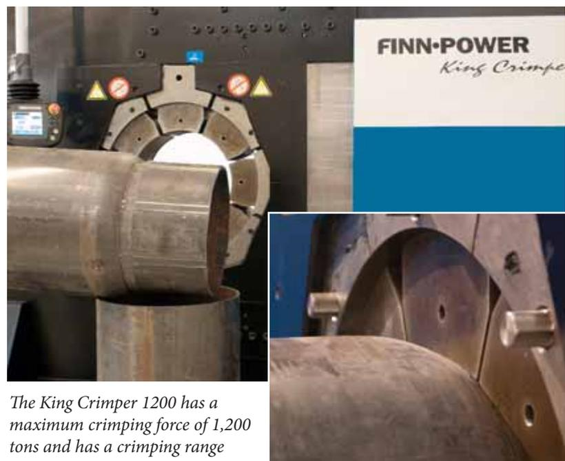
*The King Crimper 1200 has a maximum crimping force of 1,200 tons and has a crimping range from 7.87" to 25.59".*
