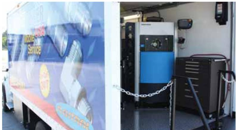
*HosePower began installing Finn-Power crimpers in its fleet of mobile service trucks in November 2009. They use the FP-120 in the large trucks and the FP-60 in the smaller vehicles.*
