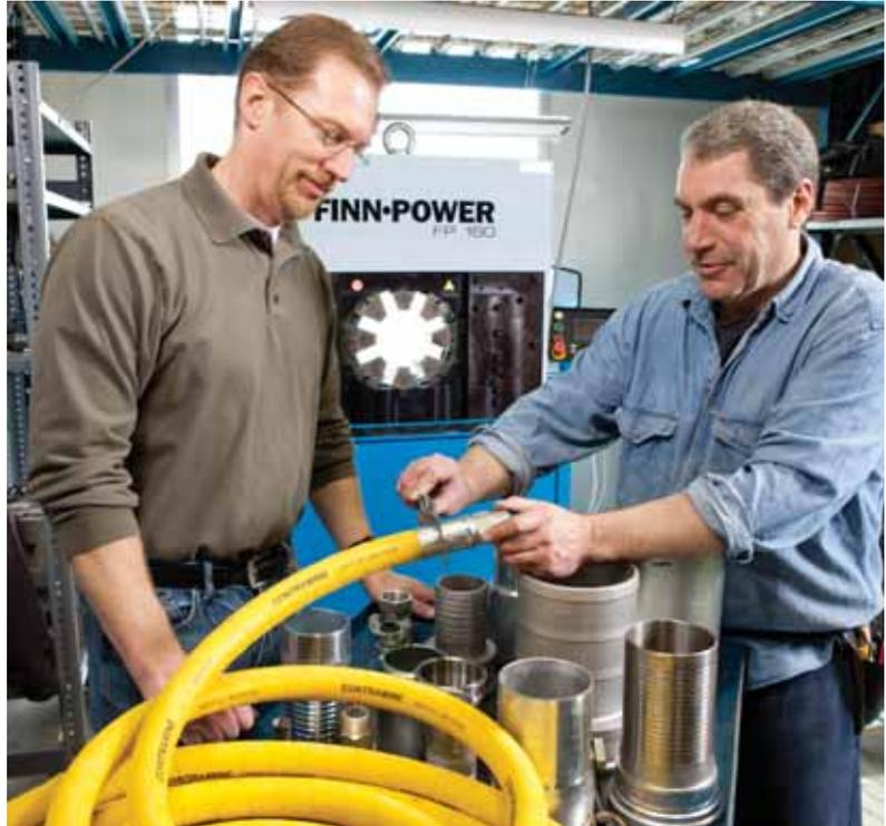
*Ted Flewwelling (left) and Steve Wickham inspect a job crimped on the FP160. IRP can now crimp from 3/16 inch ID all the way up to 6 inch ID hose with just one machine.*
