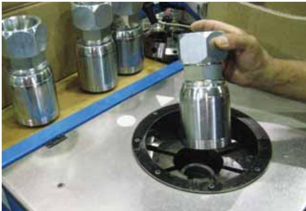
*The Finn-Power nut crimper is a very important piece of equipment at HosePower. The company crimps the nuts on all its JIC and other ring face seal nuts, as well as all the ferrules to build a one-piece fitting.*
