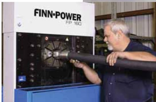
*HosePower has been using Finn-Power crimpers since 1985, and has 70 pieces of Finn Power equipment throughout its production and service facilities, consisting of hose crimpers, hose cutters, and nut crimpers. HosePower uses the FP-160 for crimping 4" hydraulic and 6" industrial hose.*
