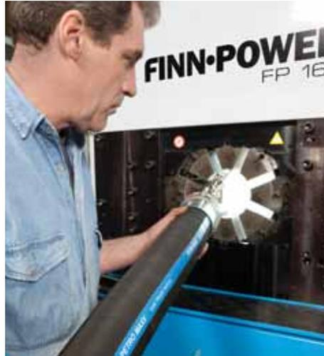
*The FP160's wide opening is also a notable feature for IRP. IRP has the ability to open the dies quite wide so that they are able to get large end fittings through it without having to worry about running the whole length through. The 6 inch capability allows the company to make assemblies that it couldn't do before.*
