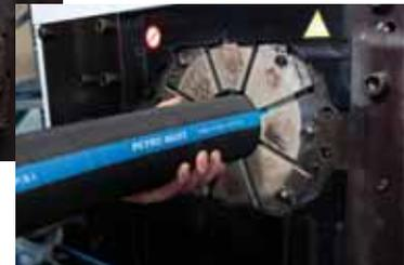
The FP160's wide opening is also a notable feature, according to Wickham. "We're not just able to do the 6 inch...we can open the dies quite wide so that we are able to get large end fittings through it without having to worry about running the whole length through," says Wickham.
